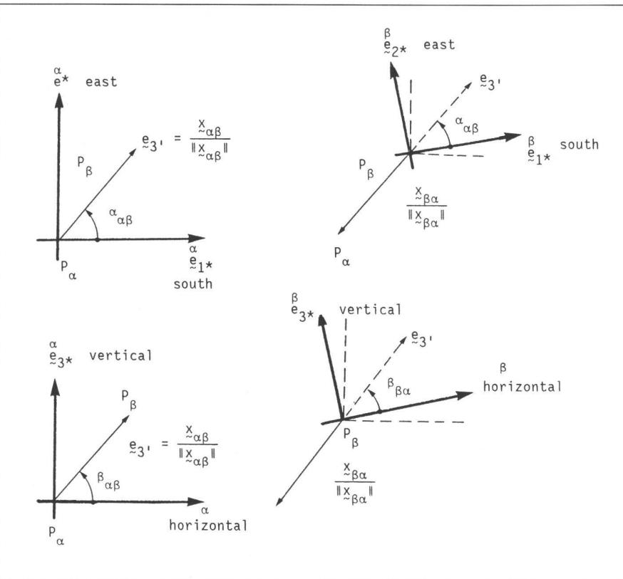
Figure A2: Horizontal and vertical projection of the Euclidean line of sight at points  $P_\alpha$  versus  $P_\beta$ , horizontal  $\alpha_{\alpha\beta}, \alpha_{\beta\alpha}$  and vertical  $\beta_{\alpha\beta}, \beta_{\beta\alpha}$  directions
