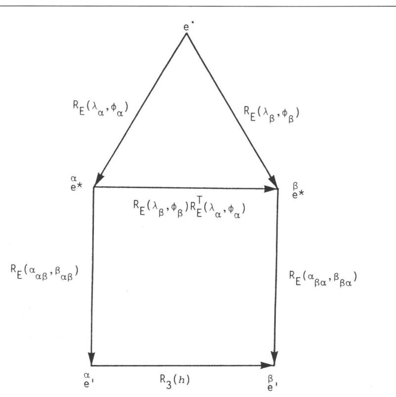
Figure A3: Commutative diagram of orthonormal triads (moving:  $e^*$ , horizontal, fixed:  $e^*$ , equatorial)
