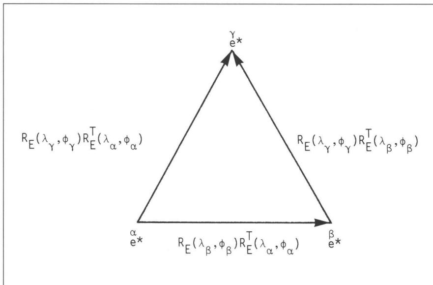
Figure 2: Commutative diagram of three orthonormal triads of horizontal type in a triangular traverse
