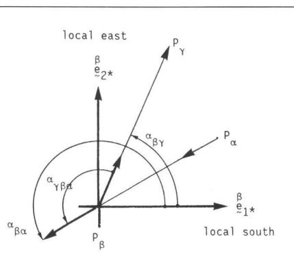
Figure A4: horizontal and vertical angles in a local horizontal triad
