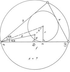
e = (f+g+h): 2 = 33.2155m $F_{\Delta} = \sqrt{e(e-f)(e-g)(e-h)} = 195.00m^2$  $R = (f \cdot q \cdot h) \cdot 4 F_{\Delta} = 13.2776 m$  $r = 2F\Delta : (f+g+h) = 5.8708m$ cos q = (f2+g2-h2):2fg, q = 44.2283 t = r: tg 9/2 = 16.216m  $y = \sqrt{R^2 - f/2)^2} = 2.701 m$  $X = \sqrt{(t-f/2)^2 + (r-y)^2} = 4.516 m$
