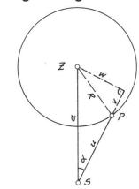
R = 24 m, q = 20.8949, a = 72 m W = a . sin q = 23.2086m  $(u+v) = a \cdot \cos \varphi = 68.1569m$  $V = \sqrt{R^2 - W^2} = 6.1124m$ u = 5 → P = 62.045m H = u · tan(+19.8529)+ I H=+21.500m
