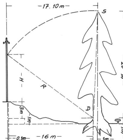
$$\begin{aligned} D + S &= R = \sqrt{20^2 + 1^2} = 20.025 \text{ m} \\ R^2 - 16^2 &= (H+3)^2 \\ \sqrt{R^2 - 16^2} &= H+3 \\ \sqrt{R^2 - 16^2} - 3 &= H = 9.042 \text{ m} \end{aligned}$$
