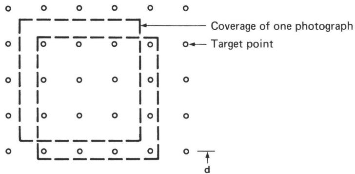
\* A passpoint is a point used to transfer geometry between adjacent photographs but is not of interest for ground location. For example, currently photogeodesy projects require placement of a single row of targets around their periphery to maintain photogrammetric geometric strength only.
