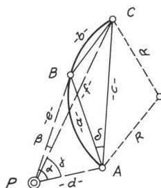
$$\begin{aligned}\alpha &= 55.455^\circ, \beta = 3.742^\circ, \gamma = 51.713^\circ \\ a &= \sqrt{d^2 + e^2 - 2de \cos \alpha} = 17.3802 \text{ m} \\ b &= \sqrt{e^2 + f^2 - 2ef \cos \beta} = 12.3804 \text{ m} \\ c &= \sqrt{d^2 + f^2 - 2df \cos \gamma} = 26.4218 \text{ m} \\ \cos \delta &= (a^2 - b^2 + c^2) : 2ac, \delta = 25.2904^\circ \\ R &= b : 2 \sin \delta = 16.000 \text{ m} *\end{aligned}$$
