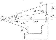
$d_{1} + g \quad \varphi = \Delta H_{1}$   $d_{1} + g \quad \beta = \Delta H_{1} + 10$   $d_{1} + g \quad \beta - d_{1} + g \quad \varphi = 10$   $d_{1} + g \quad \beta - d_{2} + g \quad \varphi = 10$   $d_{1} = 10 \cdot (f_{2} + g_{3} - f_{3} + g_{4})$   $d_{1} = 86 \cdot 188 m$   $d_{2} = d_{1} - 38 = 48 \cdot 188 m$   $H_{4} = 620 - (d_{1} + g_{3} + d_{2} + g_{3}) = 600.057 m$
