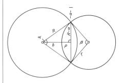
$\begin{array}{lll} p = \sqrt{R^2 - (R - a)^2 - b} & = 3.141 \text{ m} \\ r = \frac{(R - a)^2 + p/2}{2p} & = 9.371 \text{ m} \\ (R - a) : R = \sin \alpha/2, \ \alpha & = 98.727^9 \\ (R - a) : r = \sin \beta/2, \ \beta & = 107.400^9 \\ F = [R^2 (arc \ \alpha - \sin \alpha) + r^2 (arc \ \beta - \sin \beta)] : 2 \\ F = 58.0 \ m^2 \end{array}$
