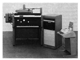
Abb. 10 Orthophotosystem Avioplan OR1
