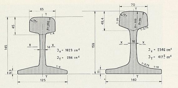
Links: Schienenprofil SBB I 45,93 kg/m
