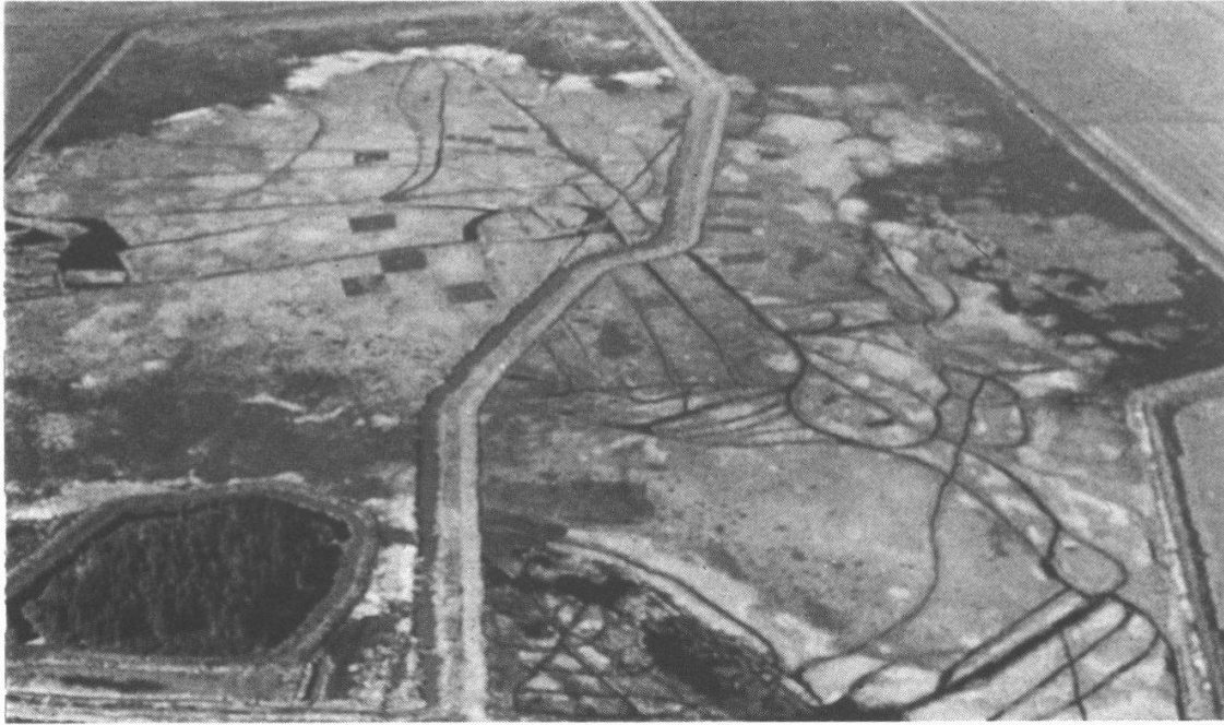
Fig. 2. Aerial view of the study area: The photograph shows the Hog Lake Impoundment in 1981, with the central dyke dividing the impoundment into an undrained (on the right hand side) and a drained basin (on the left hand side). The "trails" were mechanically cut through the floating mat to improve the area for waterfowl. Rectangular dark areas are burned plots.
