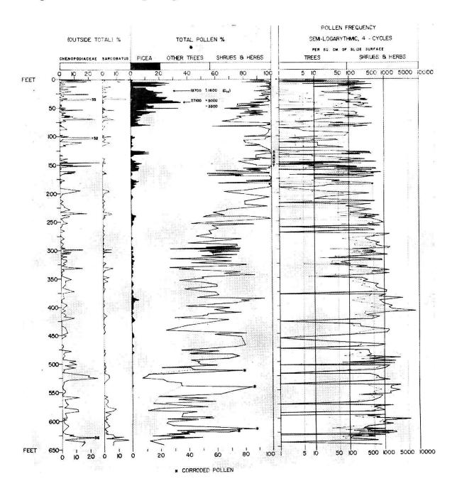
Pollen frequency has been plotted on a semi-logarythmic curve per sq. cm. of slide surface. Sediment horizons with no pollen include oxidized zones, silt and clay free sands, and soils.
