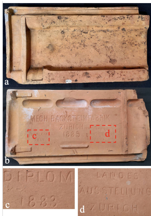
Figure 5.9: Uppside (a), underside (b) and two enlarged areas (c, d) of the intact tile ZZ 448 (Dimensions 420 × 225 × 30 mm), showing three impressed inscriptions. In the centre «MECH. BACKSTEIN- FABRIK / ZÜRICH/1885» (Height of the letters: 20 mm, of the numbers 1 and 8: 17 mm, of the number 5: 18 mm), below left (c) «DIPLOM/1883» and right (d) «LANDES/AUSSTELLUNG/ZÜRICH» (Height of the letters: 7 mm). A raised mark in the form of an inverse italic Roman number two below the large central inscription («||», height 12 mm) can be seen. Photos MARINO MAGGETTI.
