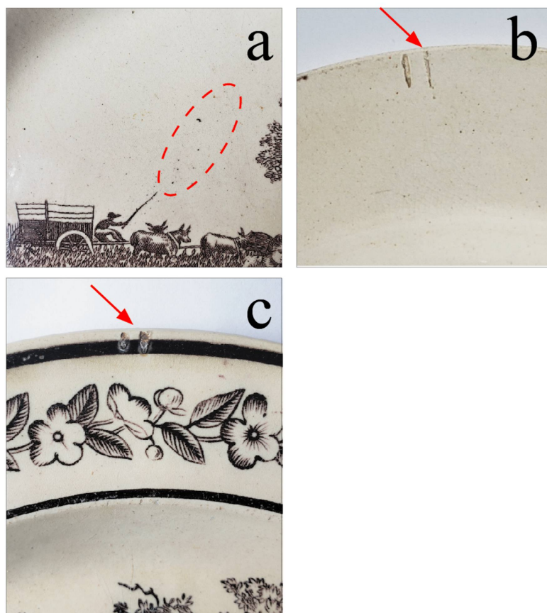
Figure 9.11: Distinguishing criteria found on some white earthenware attributed to « Geneva-La Balme ». (a) Unwanted dusting of metal oxides in the red dotted oval, not cleaned before applying the glaze. 7x5 cm. VALFRÉ coll. no 3; Traces left by the firing supports visible not only on the reverse (b) but sometimes also on the obverse (c). 5x7 cm. VALFRÉ coll. no 8, « Gesler demande pourquoi cette seconde flèche ... » [Gesler asks why this second arrow ...]. Photos PATRICE VALFRÉ.
