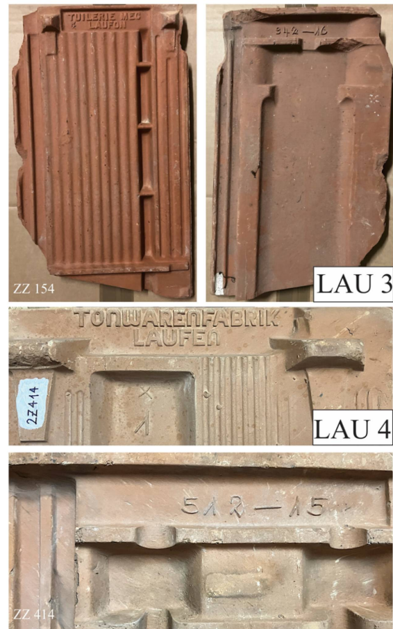
Figure 8.21: LAU 3: ZZ 154 (Image widths 16.7 cm) with mark on the underside (H letters 1.0 cm) and production date on the outside (H numbers 1.2 cm). LAU 4: ZZ 414 with mark (Image width 18.3 cm; H letters 0.8 cm; H numbers 0.9 cm) and production date on the outside (Image width 18.6 cm; H numbers 1.1–1.3 cm). Photos MARINO MAGGETTI.
