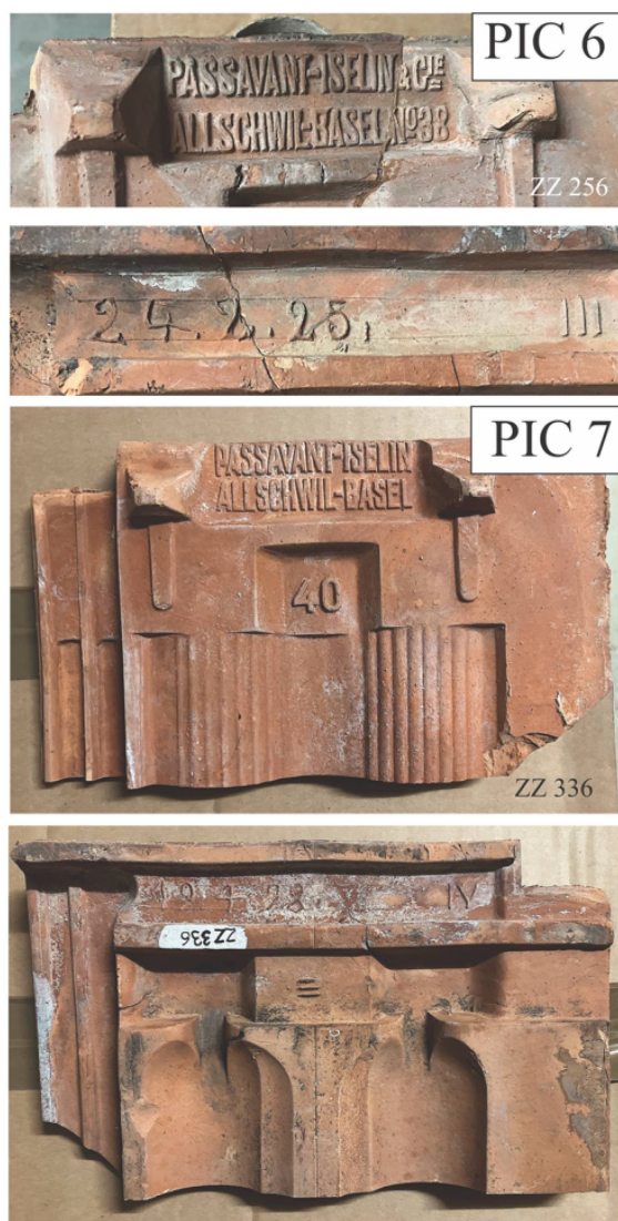
Figure 8.16: PIC 6: ZZ 256 with mark (Image width 17 cm; H letters 1.3 cm) and production date (Image width 16 cm; H numbers 1.2 cm). PIC 7: Under- and outside (Image widths 25 cm) of ZZ 336. Mark on the underside (H letters 1.3 cm; «40» 1.6 cm) and the production date on the outside (H numbers 1.5 cm). Photos MARINO MAGGETTI.
