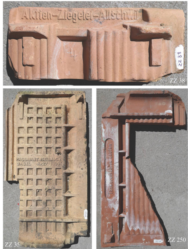
Figure 8.10: The three possible positions of the stamped marks on the undersides of the studied roof tiles. ZZ 38 (AZA) 20 × 8.5 cm ; ZZ 35 (PIC) 42 × 23 cm; ZZ 250 (Laufen) 42.5 × 17.5/24 cm. Photos MARINO MAGGETTI.
