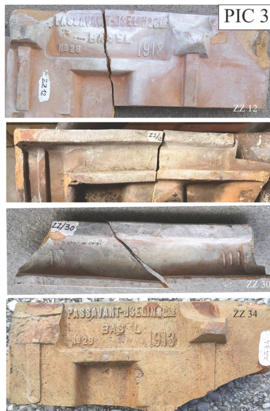
Figure 8.12: PIC 3: Under- and outsides of ZZ 12 with the mark and the production date (Image width 19.5 cm; H letters 0.8 cm; H numbers 1.2 cm). Outside of ZZ 30 with badly readable production date (Image width 16 cm). Underside of ZZ 34 with the mark (Image width 20 cm; H letters 0.8 cm; H numbers on the right 1.2 cm). Photos MARINO MAGGETTI.
