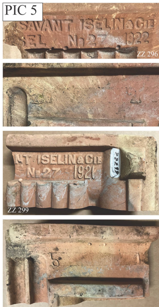
Figure 8.15: PIC 5: Under- and outside (Image widths 12 cm) of ZZ 296 (H letters and numbers 0.8 cm; outside: H numbers 1.2 cm) and ZZ 299 (Image widths 13.3 cm) with the mark (H letters 0.8 cm; year numbers 1.1 cm) and the production date (H numbers 1.2 cm). Photos MARINO MAGGETTI.
