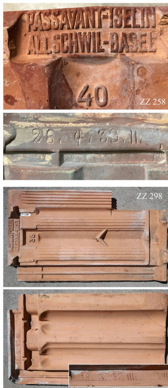
Figure 8.17: PIC 7: Under- and outside (Image widths 10.5 cm) of ZZ 258 with mark on the underside (H letters 1.3 cm; «40» 1.5 cm) and production date on the outside (H numbers 1.1 cm). ZZ 298 (40 × 24 cm) with the marked underside (H letters 1.3 cm; «38» 1.4 cm) and the outside with the production date (H numbers 1.1 cm), see also the cutout. Photos MARINO MAGGETTI.
