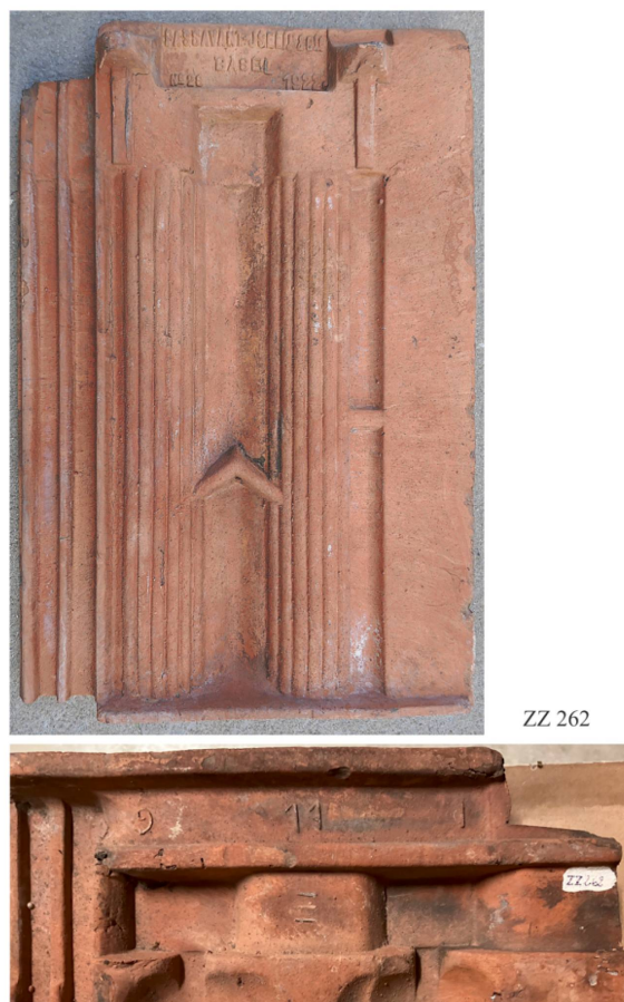
Figure 8.13: PIC 3: Under- (36 × 24 cm) and outside (Image width 22 cm) of ZZ 262 with the mark (H letters 0.9 cm) and the production date (H numbers 1 cm). Photos MARINO MAGGETTI.
