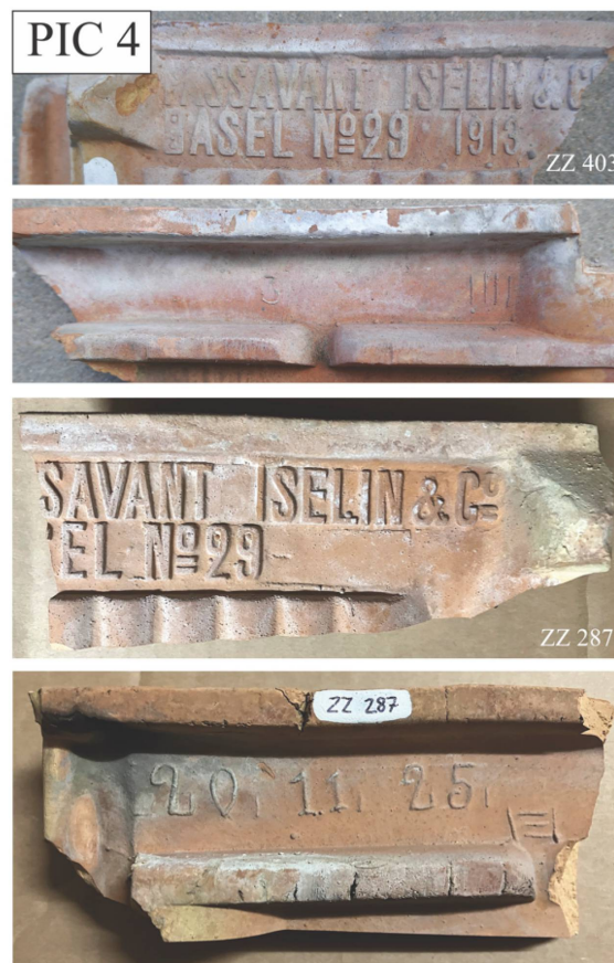
Figure 8.14: PIC 4: Under- and outside (Image widths 20 cm) of ZZ 403 and ZZ 287 (Image widths 14 cm) with the mark and the production date. Height of the letters and numbers 1.5 cm. Photos MARINO MAGGETTI.
