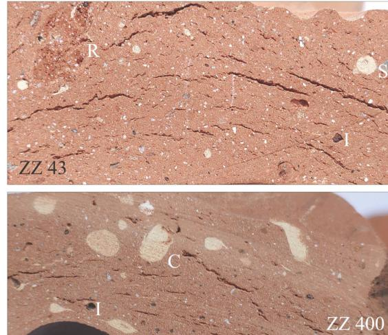
Figure 8.25: *Macroscopic aspects of typical roof tiles from Laufen. ZZ 43 = texture I, ZZ 400 = texture II. Sawn sample area, image widths 4 cm. C = carbonate grain, I = iron-rich clay nodule, R = relic of the Ca-poorer raw material, S = sandstone grain. Photos MARINO MAGGETTI.*
