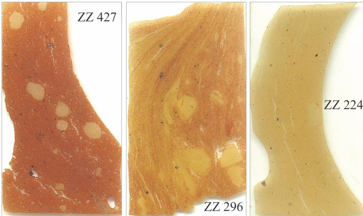
Figure 8.26: *Scans of three typical thin sections with the transition from a heterogeneous texture II (ZZ 427) via a streaky texture II (ZZ 296) to a homogeneous texture I (ZZ 224). Respective image width: 2 cm. Scans MARINO MAGGETTI.*
