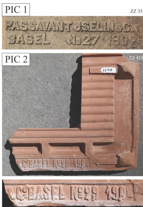
Figure 8.11: *PIC 1: Underside of ZZ 35, showing the mark (Image width 13.5 cm; height (H) of the letters 0.9 cm). PIC 2: Underside of ZZ 418 (24.5 × 23 cm) with enlarged view of the mark (Image width 15.5 cm; H letters 1.6 cm).* Photos MARINO MAGGETTI.
