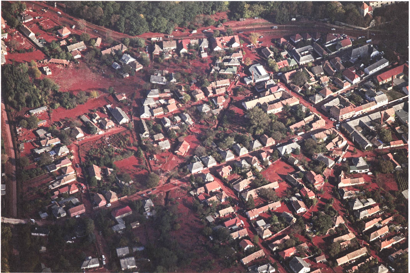
5 The dyke around a red mud basin in Ajka, Hungary, collapsed in 2010, causing the toxic sludge to flood an extensive area, killing 10 people.
