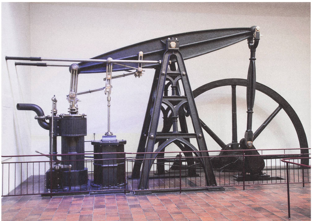
2 Top: Replica of the Boulton & Watt "Lap engine" (1788), built by the Eisenbahnausbesserungswerk, Munich, 1913 (Inv. No. 37193). Bottom: First steam engine installed at the Krupp firm, made by the Hüttengewerkschaft Jacobi, Haniel & Huyssen (later Gutehoffnungshütte), Sterkrade, 1835 (Inv. No. 2348).
