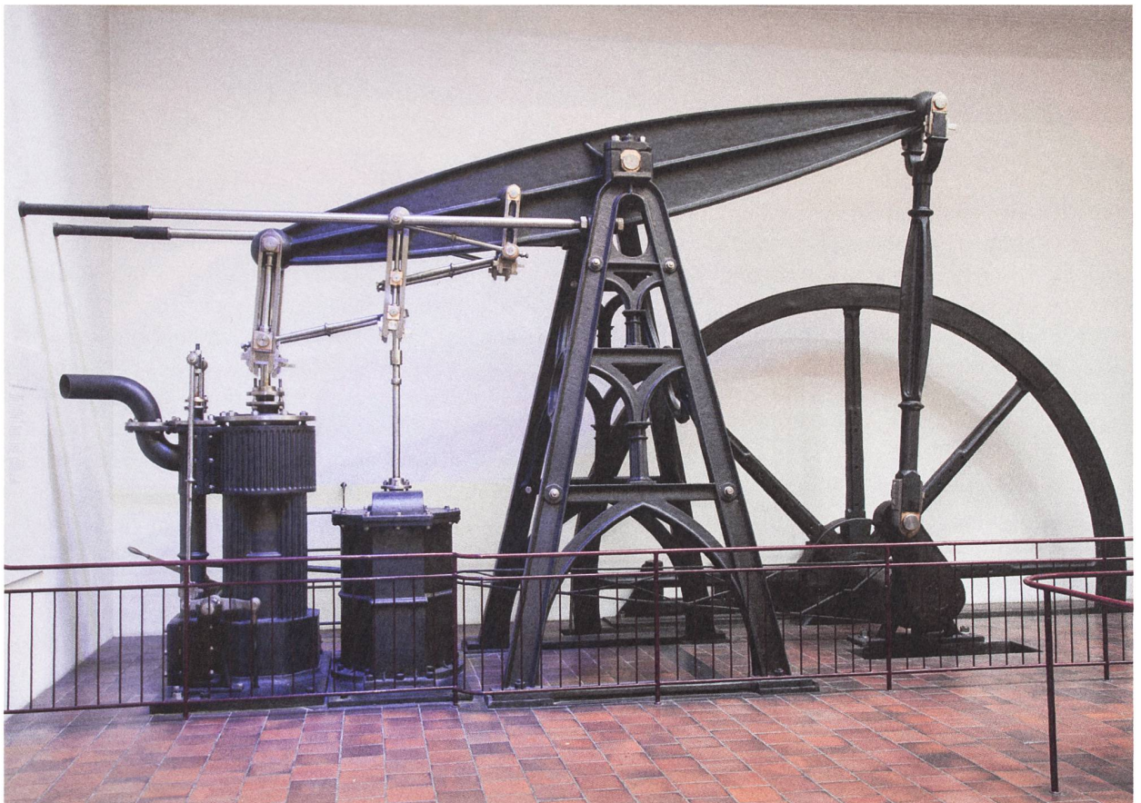
2 Top: Replica of the Boulton & Watt "Lap engine" (1788), built by the Eisenbahnausbesserungswerk, Munich, 1913 (Inv. No. 37193). Bottom: First steam engine installed at the Krupp firm, made by the Hüttengewerkschaft Jacobi, Haniel & Huysen (later Gutehoffnungshütte), Sterkrade, 1835 (Inv. No. 2348).
