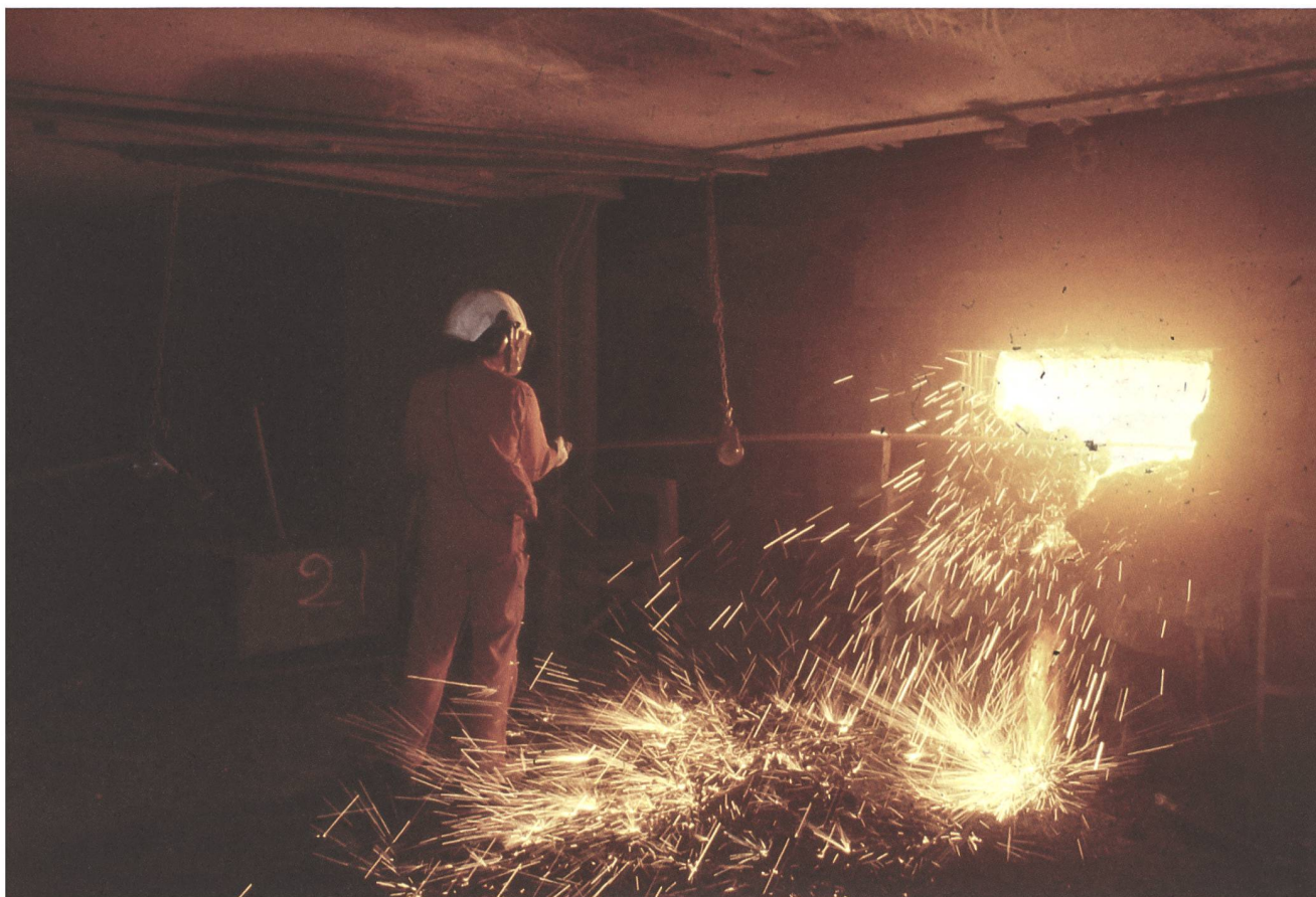
6 Samples are taken from the electric arc furnace, 1990.
