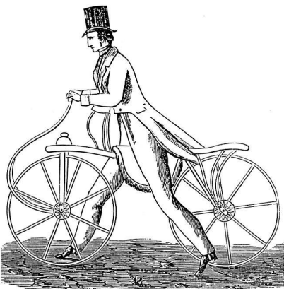
Bild 11: Draisine von Denis Johnson, Long Acre «in the county of Middlesex, coach maker» (British Patent 1818). Aus: The Engineer ; vol. 27, 1869, p. 197.
