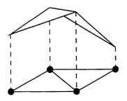
In this way the graph becomes the surface of a convex mountain. The graph is flat (but not necessarily horizontal) over a rhombus if and only if the rhombus inequality is satisfied with equality.
