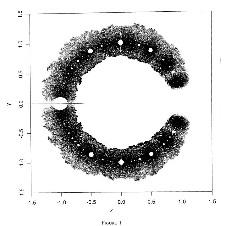
Scatterplot of zeros z = x + iy of polynomials of degrees  $\leq 16$  with constant term 1 and coefficients 0 and 1. The "segments" along the negative real axis are created by negative real zeros. Negative real zeros < -1.5 are not shown.
