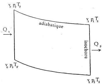
$$\begin{array}{c} \text{Fig. 3.} \\ \text{isochore} : \frac{p_2}{p_1} = \frac{T_2}{T_1} \ ; \\ \text{adiabatique} : \left(\frac{v_0}{v_1}\right)^{k-1} = \frac{T_1}{T_0} \ , \quad \left(\frac{p_1}{p_0}\right)^{\frac{k-1}{k}} = \frac{T_1}{T_0} \ ; \end{array}$$
