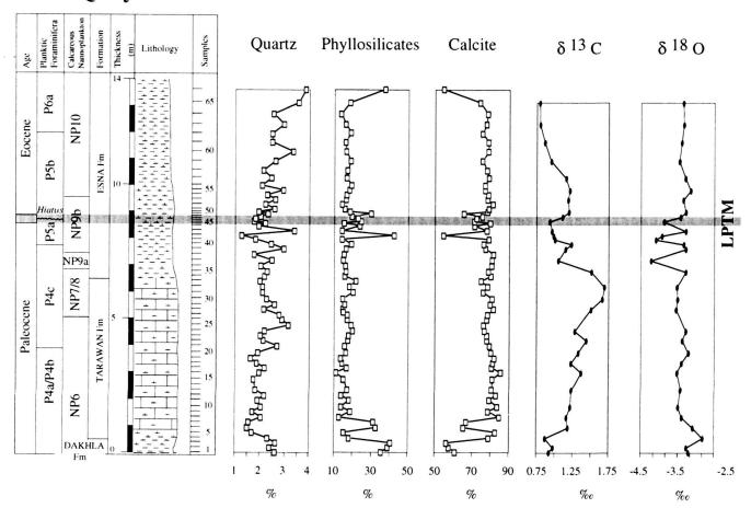
Fig. 5. Bulk rock mineral compositions and stable isotopic trends at Gebel Qreiya. Stable isotopes analyses were conducted on the fine fraction ( $< 63 \,\mu m$ ) of the bulk samples. See Fig. 2 for symbol explanation.
