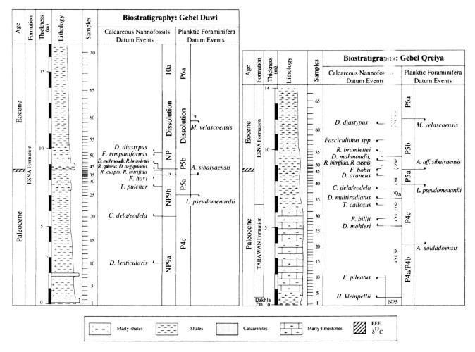
Fig. 2. Lithologic log with sample locations and biostratigraphic zonations of the Gebel Duwi and Gebel Qreiya sections, central Eastern Desert. LPTM = Late Paleocene Thermal Maximum interval.
