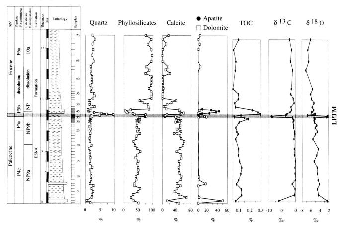
Fig. 4. Bulk rock mineral compositions, total organic content (TOC) and stable isotopic trends at Gebel Duwi. Stable isotopes analyses were conducted on the fine fraction (< 63 µm) of the bulk samples. See Fig. 2 for symbol explanation.
