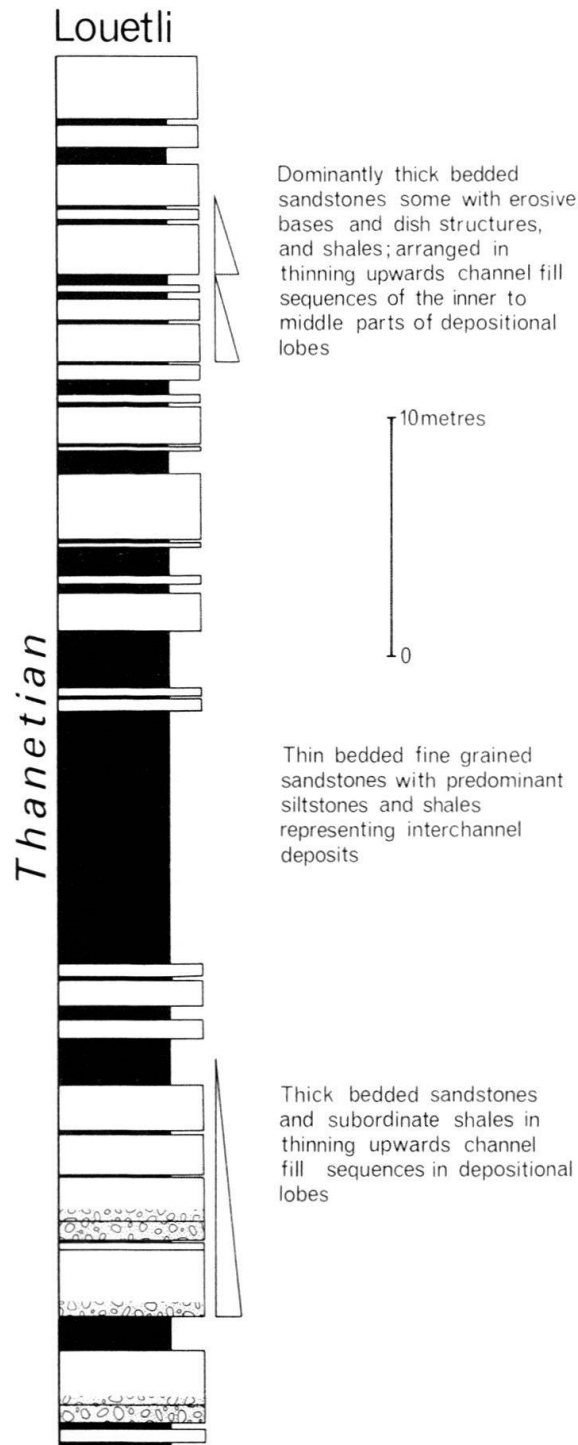
Fig. 6. Log of the section of the Gurnigel flysch exposed in the Louetli quarry.
