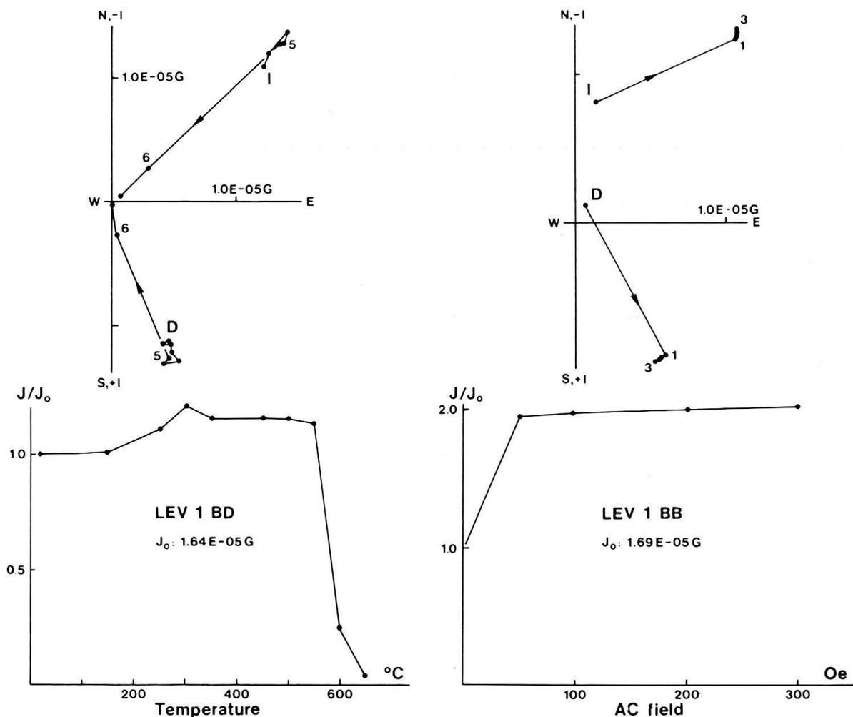
Fig. 3. Thermal and *AF* demagnetization of *NRM* of high coercivity samples. *NRM* intensity decay during demagnetization plotted on the lower two diagrams. *NRM* directional variations given as projections of the declination and inclination components of *NRM* in the upper two vector plots.
