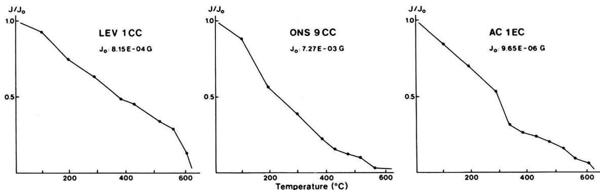
Fig. 2. Progressive thermal demagnetization of *IRM* acquired in a field  $H = 8$  kOe. The different shape of the demagnetization curves and the different maximum blocking temperatures indicate the presence of several ferromagnetic minerals.
