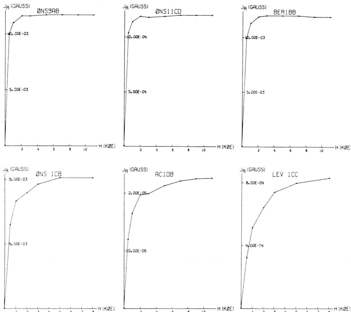
Fig. 1. Two types of *IRM* acquisition curves are observed in the Lepontine metamorphic rocks. Upper series saturates below  $H=2$  kOe; lower series contains ferromagnetic minerals with coercivities greater than 2 kOe.
