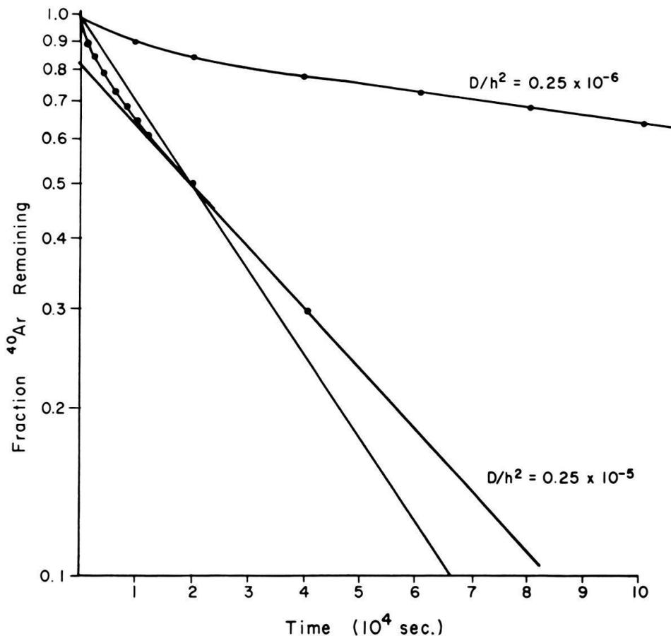
Fig. 2. Fraction of argon remaining in a slab according to rigorous solution and exponential approximations. The two diffusion curves represent a temperature difference of about  $75^\circ\text{C}$ . The error in using the exponential approximation is equivalent to a temperature difference of not more than approximately  $10^\circ\text{C}$ . The  $D/h^2$  curves were calculated by LAUGHLIN (1969).
