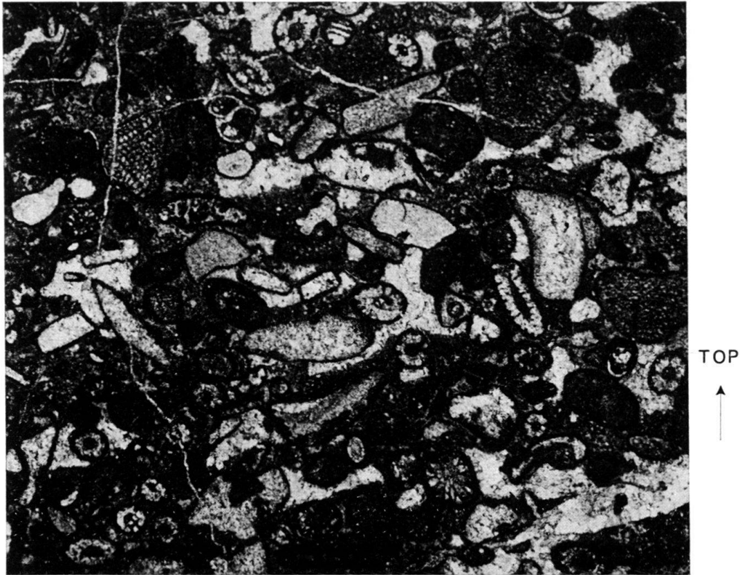
Fig. 7. Schrattenkalk: skeletal lime grainstone (packstone) . The grains are not too well sorted and are superficially coated. Note the internal sediment which floors the pore space. The grains are made up mainly of recrystallized, mollusc and probably coral fragments. There are abundant sections through dasyclad algae ( Salpingoporella ), bryozoans, echinoderm fragments and worn conical orbitolinids. This type of sediment, in close connexion with the previously described (Fig. 6) overlying sample, could be expected in a beach complex periodically exposed to vadose conditions. Environment: normal marine high energy bar complex. Section No. 2, Habernlegi, Acetate peel, 10 \times .
