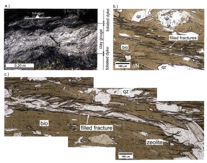
Fig. 9. a) Photo of clayey-sandy fault gouge within a sheared heavily foliated lamprophyric dyke. b) Microscopic view of a foliated lamprophyric dyke, showing enechelon micro-fractures filled with zeolites. c) Large micro-fracture within lamprophyric dykes, aligned parallel to foliation and suggesting tensile opening.
