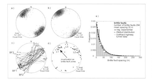
Fig. 4. a) Brittle fault zones mapped within the Gotthard safety tunnel. b) Brittle fault zones mapped on surface (plotted as poles). c) Brittle fault zones mapped on surface with measured slickenside striations and shear sense indicators. d) Orientation of intrusion contacts for the lamprophyric dykes (plotted as poles). e) Total spacing histogram of brittle fault zone measured within the Gotthard highway safety tunnel.
