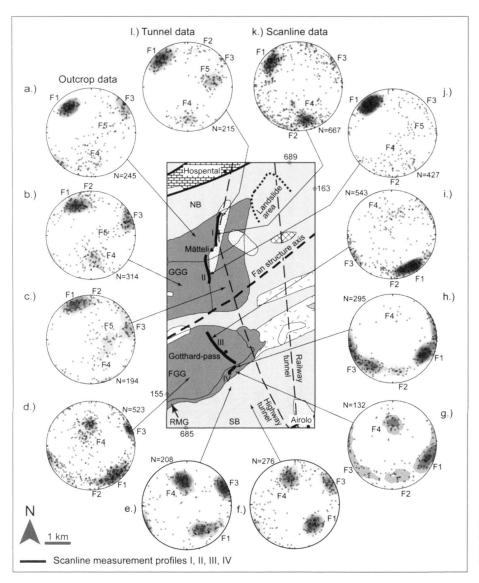
Fig. 13. Location and orientation of joints that are sampled on surface and within the Gotthard highway safety tunnel (l) through outcrop (a-g) and scanline (h-k) measurements. See Fig. 2 for legend.
