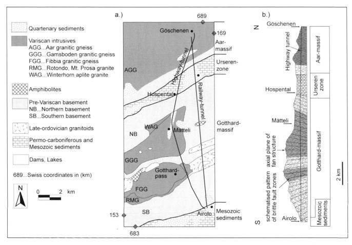
Fig. 2. a) Geological overview of the study area. b) Cross section along the Gotthard highway tunnel showing geological and tectonic units (modified after Keller et al. 1987). Within the Gotthard massif a schematised pattern of foliation and brittle fault zones (i.e. the fan structure) is shown.
