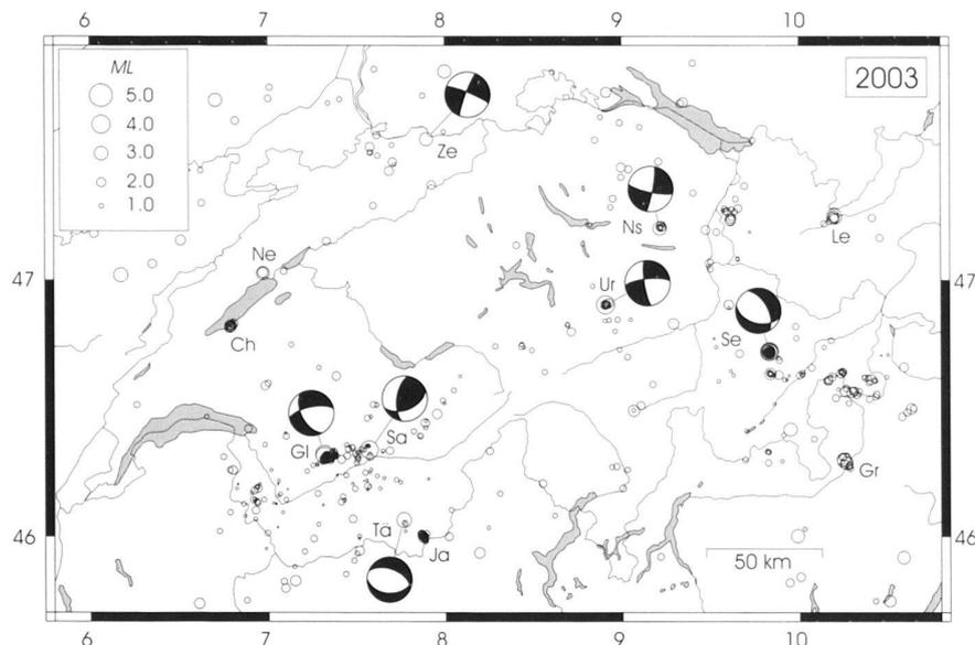
Figure 2. Epicenters and focal mechanisms of earthquakes recorded by the Swiss Seismological Service during 2003. Epicenters of earthquakes mentioned in the text are Cheyres (Ch), Glarey (Gl), Grosio (Gr), Cima di Jazzi (Ja), Lech (Le), Neuchâtel (Ne), Nesslau (Ns), Salgesch (Sa), Sertig (Se), Täsch (Tä), Urnerboden (Ur), Zeiningen (Ze).
