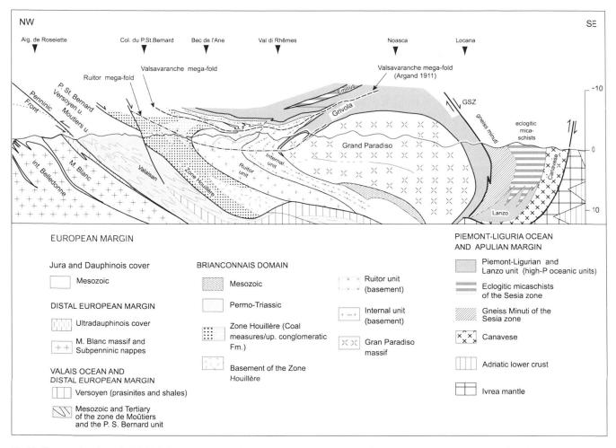
Fig. 13. Cross section along the ECORS-CROP seismic line (profile trace indicated in Figs. 1 & 2), modified after Schmid & Kissling (2000), depicting two large-scale post-nappe folds at the scale of the orogen. GSZ: Gressonney shear zone.
