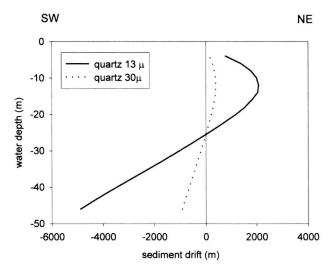
Figure 6. Particle trajectories along a NE-SW plane in a water column of 5  $^{\circ}$ C, calculated for the event of «vent» from 24 - 28 October 1998 (Fig. 3a). Trajectories have been calculated at the site of the current meter using Stokes law for quartz particles of 13 and 30  $\mu m$  in diameter and homogenous mean current velocity for 2-m depth intervals.
