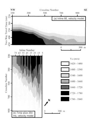
Fig. 2. Model of stacking velocities ( $V_{st}$ ) along (a) inline 66 and (b) time slice at 350 ms for all 80 navigated lines. See Figs. 1 and 3 for location.
