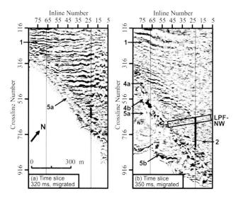
Fig. 4. Selected migrated time slices from 3-D survey: (a) time slice at 320 ms and (b) time slice at 350 ms. Interpretation: 1 - Plateau Molasse, 2 - deformed Subalpine Molasse, 4a/4b - glacial sediments, 5a/5b - post-glacial sediments and LPF-NW - northwest fault of La Paudèze thrust zone. Vertical lines show inline location (Figs. 2 and 3), and thickened portions indicate extent of facies 2. See Fig. 3 for time slice location.
