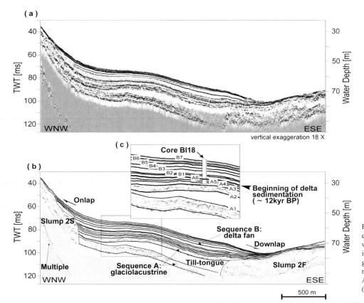
Fig. 4. (a) uninterpreted, (b) interpreted echosounder profile IB05 with enlarged window showing BI18 coring site (c). As indicated by downlap termination on glacio-lacustrine sequences, the delta sedimentation begun at around 12 kyr BP. Ages are obtained from the core BI18 (Fig. 5). Refer to Fig. 1 for location.
