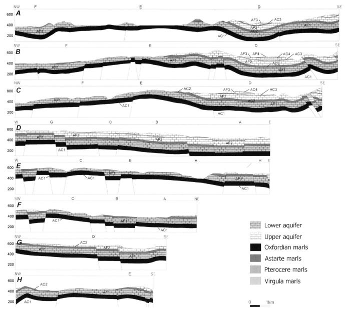
Fig. 5. Hydrostratigraphic cross sections. Hydrostartigraphic units are labeled with their codes for orientation. Vertical exaggeration is 2.5.
