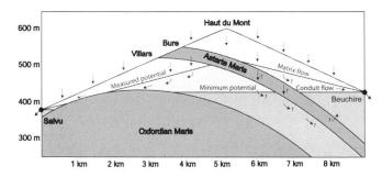
Fig. 13. Conceptual model of the Bure aquifer. This N-S oriented theoretical cross section between Boncourt and Courtedoux shows the minimum estimate of the hydraulic heads in the karst conduits (assuming zero hydraulic gradient) and the mean water table (obtained from piezometers). Arrows indicate flow directions.
