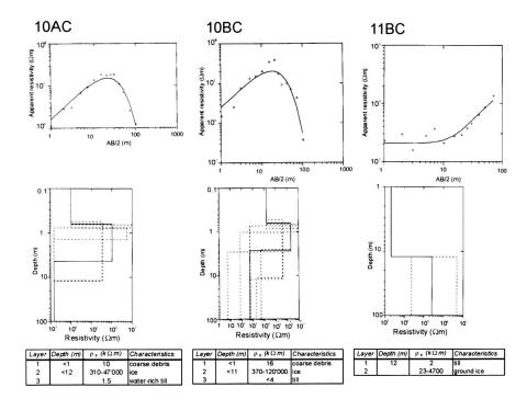
Fig. 5. Examples of DC data (for locations of G10 and G11 see Fig. 2A). Upper panels: Open circles are measured data points, the black line is the calculated fitting curve. Middle panels: The calculated equivalent layer models. The mean resistivity model (solid line) was chosen for further interpretation and Tab. 3. The tables give the depth and resistivity ranges of the computed possible layer models. 10AC and BC are the Hummel branches at sounding point G10.
