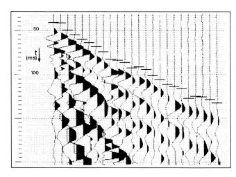
Fig. 3. Example of a seismogram section (shot 5 in Fig. 4A). Horizontal marks are the first arrival picks as used for the time-distance plots. This record section led to the following velocities:  $v_1$ = 700 m/s (shotpoint to geophone 5);  $v_2$ = 1300 m/s (geophone 5 to 24). Note that this figure shows travel time versus geophone number, not versus distance. The equal geophone distances in the figure are given by the plotting instrument. Uphill direction is on the right-hand side.
