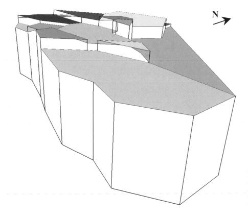
Fig. 8b. Three dimensional view of the disturbing body obtained by a combined interpretation of the airborne and ground residual anomalies. The colours are of arbitrary choice and serve only to facilitate the understanding the three dimensional character of the body.
