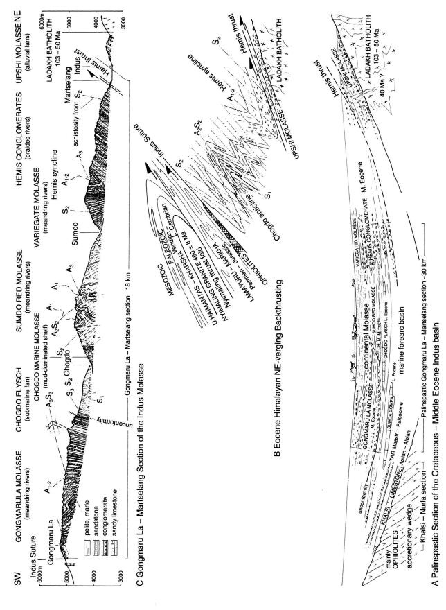
Fig. 5. Geological section of the Gongmarula-Martselang transect through the Indus Molasse (C), the Eocene phase of NE-verging (back) thrusting (B) and the palinspastic section of the Upper Cretaceous – Middle Eocene Indus basin (A) according to Steck et al. (1993).
