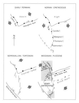
Fig. 10. Summary of structural evolution of the western termination of the Valsugana Line from the Early Permian to the Pliocene. Paleogene extensional tectonics is omitted, although some Paleogene oblique extension reactivated pre-existing N-S trending faults.
