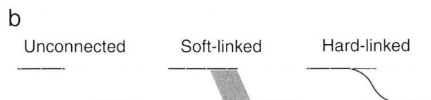
Fig. 1. Schematic diagram illustrating: (a) contractional and extensional steppovers and bends occurring in a strike-slip fault system with sinistral kinematics, (b) evolution of a growing strike-slip fault from two unconnected segments to a single fault with a double bend.
