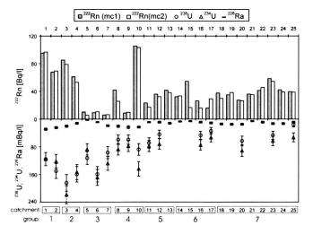
Fig. 4.  $^{222}$ Rn concentrations of water (1  $\sigma$  error: 8% for < 10 Bq/l, 4% for > 10 Bq/l) sampled during 2 measuring campaigns (mc 1, mc 2), and  $^{238}$ U,  $^{234}$ U and  $^{226}$ Ra concentrations (with 2  $\sigma$  error bars) from mc 1.
