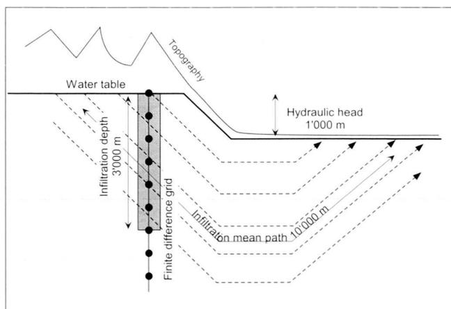
Fig. 7. Description of the thermal model. The fixed grid-nodes are shown, while geological limits are moving through these grid points. The shaded area indicate the zone influenced by water circulation. The schematic flow lines have an average length of 10'000 m.
