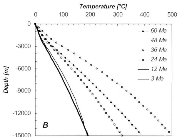
Fig. 10. Evolution of the depth-temperature profiles with time for an infiltration mean-path of  $10^4$  m as was considered in the models described in figures 7 and 9. A) Purely conductive model. B) With water circulation for a hydraulic conductivity of  $2.5 \times 10^{-9}$  m/s.
