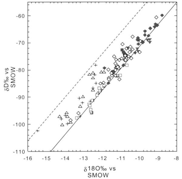
Fig. 4.  $\delta D$  vs.  $\delta^{18}O$  diagram. Full line = Worldwide meteoric water line (Rozansky et al. 1993); dash line = Mediterranean meteoric water line for a deuterium excess of 220 (Vuataz 1982). The plotted points represent cold and warm springs as well as water inflows in Alpine tunnels. Data from Pastorelli (1999) with the exception of the isotopic values of the springs and the water inflows in the Simplon region, which are taken from Martinotti et al. 1999.
