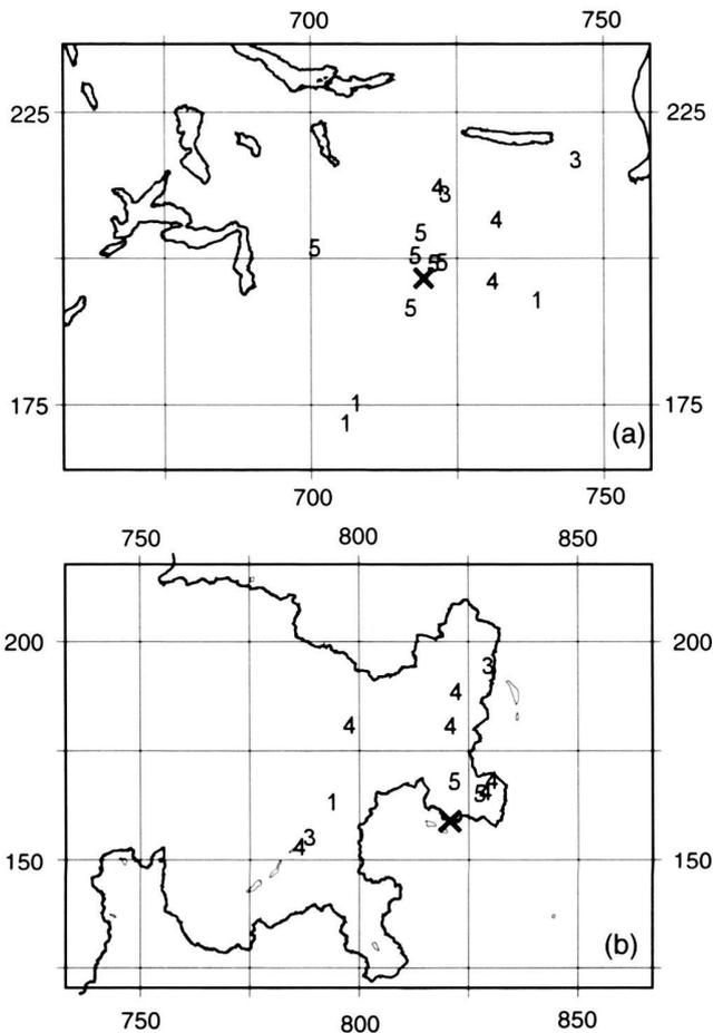
Fig. 5. Macroseismic observations of the Linthal event of 2001/03/17 (a) and of the Bormio event of 2001/10/01 (b). Each value represents the macroseismic intensity (EMS-98) assigned to a single postal code zone. The X corresponds to the instrumental epicenter. The Swiss cartesian coordinate grid is labeled in km.
