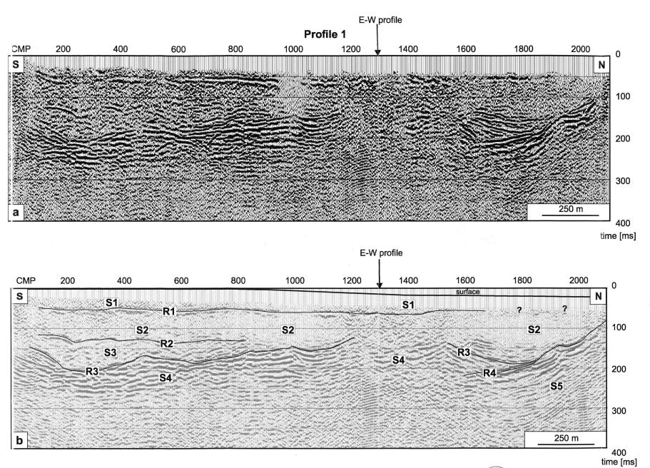
Fig. 6. (a) stacked section of Profile 1 (north-south profile). Note changes in amplitude character with increasing two-way traveltime. (b) Migrated section of (a) with interpreted units and main reflectors. Arrow on top marks the intersection with Profile 2 (E-W profile). For identification of units see text and Fig. 8.
