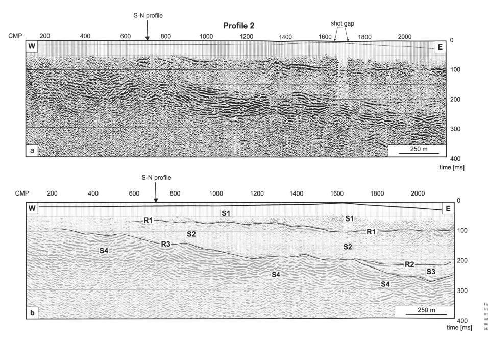
Fig. 7. (a) stacked section of Profile 2 (east-west profile). Note changes in amplitude character with two-we traveltime as in fig. 6a. (b) Migrated section of (a) will interpreted units and main reflectors. Arrow on wrarks the intersection with Profile 1 (S-N profile). Fridentification of units see text and Fig. 8.
