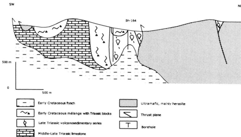
Fig. 6. Cross-section of Rubiku area, showing thrusting of Upper Triassic limestone-volcanosedimentary and ultramafic rock association onto the Jurassic-Cretaceous flysch.
