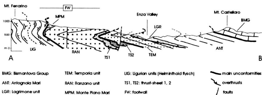
Fig. 3. Geological cross-section across the thrust system of the Enza Valley. For location see figure 2
