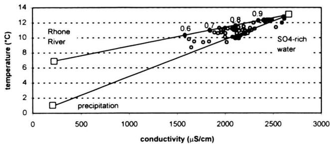
Fig. 7. Correlation between electrical conductivity and temperature of Q6 spring for the observation period from April 14 to May 6, 1998 (measure interval = 3 h). The four black dots represent simulated mixing proportions from 0.6 to 0.9 between the Rhone River and SO<sub>4</sub>-rich water.
