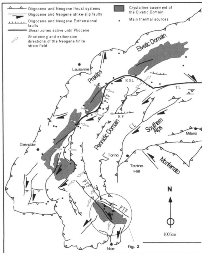
Fig. 1. Tectonic sketch map of the Western Alps. Dark shadowed areas are the External crystalline Massifs (European continental crust). Dots are the most important thermal springs. RSL = Rhône-Simplon Line, TL = Tonale Line, PTF = Penninic Thrust Front, RF = Ranzola Fault.
