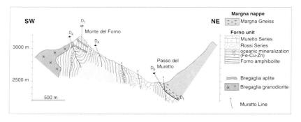
Fig. 12. Section across the Forno and the Margna units at Passo del Muretto showing the occurrences of Fe-Cu-Zn mineralizations.
