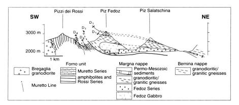
Fig. 3. Detailed SW-NE section through the eastern margin of the Bregaglia pluton (after Spillmann 1993).
