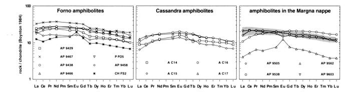
Fig. 15. REE patterns of Forno amphibolites, Cassandra amphibolites and Margna amphibolites. REE pattern of Margna amphibolites from Bissig (1997) is given for comparison (shaded area). Normalization on an average CI chondrite (Boynton 1984).
