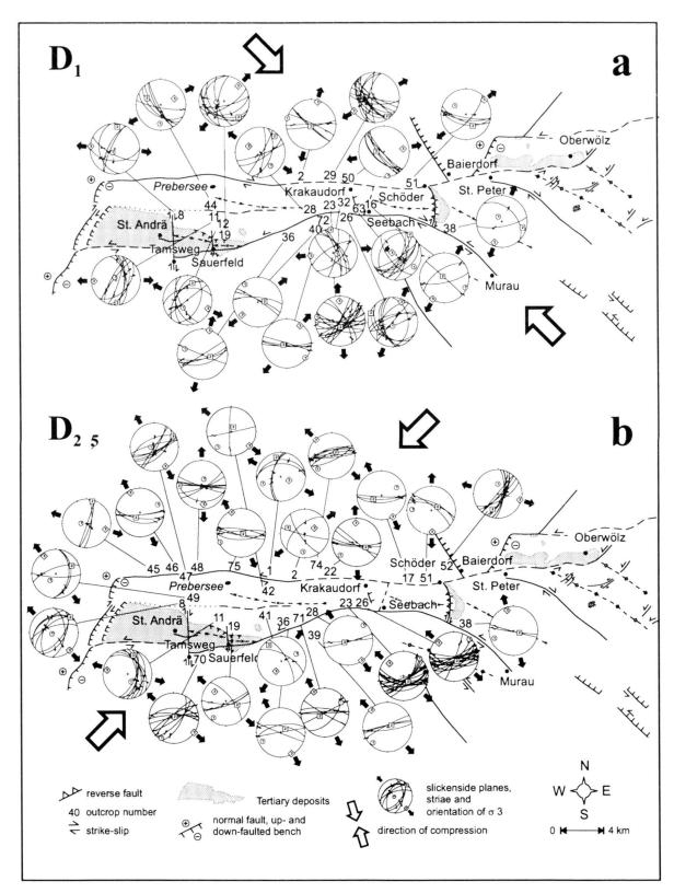
Fig. 5. Palaeostress patterns of deformation stages (a)  $D_1$  dextral strike-slip regime with NW-SE orientation of the maximum principle stress axis, and (b) combined  $D_2/D_5$  sinistral strike-slip with NE-SW orientation of the maximum principal stress axis.
