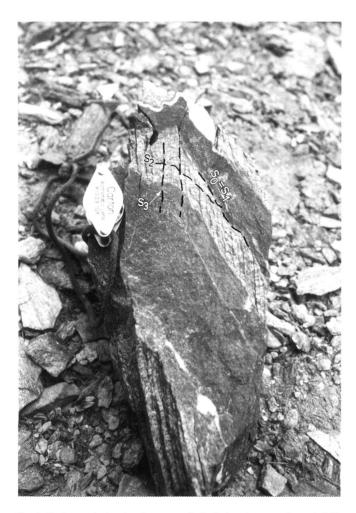
Fig. 4. Rock sample showing the geometrical relations between the main foliations. S2 intersects at low angle the lithological bedding (S0). These are both deformed by later folds that develop a crenulation cleavage here indicated as S3.
