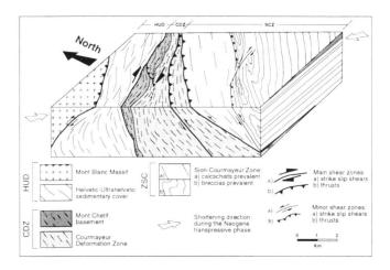
Fig. 12. Schematic block diagram of the study area representing the main structural features related to progressive Neogene transpressive tectonics.
