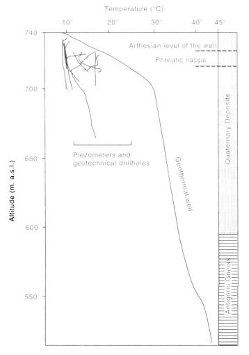
Fig. 10. Temperature logs measured in geotechnical drill-holes already present in the Piedilago area.
